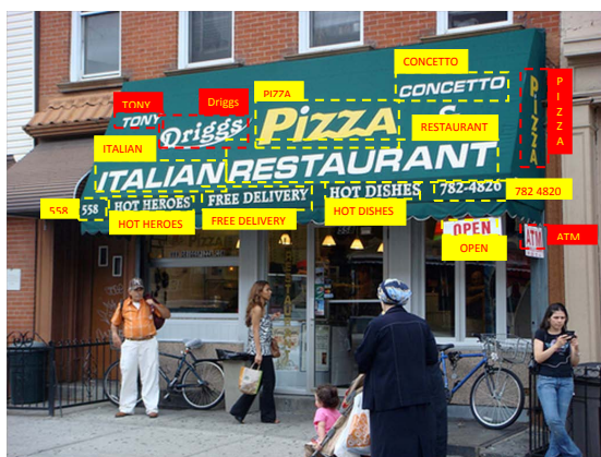
Fig. 7. Yellow dashes and boxes denote our output. The red boxes are not recognized.
