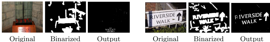
Fig. 4. System output illustrating robustness to highlights and shadows.
